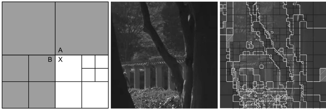
Fig. 2. Left: schematic representation of a current block X , its set of merging candidates \{A, B\} , and its causal neighborhood (gray shaded). Middle: cropped part ( 512 \times 512 ) of a frame of the 1080p test sequence ParkScene . Right: illustration of MCP blocks (black lines), merged regions of MCP blocks (white lines), and intra-coded blocks (striped pattern) for the same cropped ParkScene content. With a chosen CTB size of 64 \times 64 , an area covering 64 CTBs is shown. Note that ParkScene contains a scene captured using a laterally from left to right moving camera and thus, the trees in the foreground, as shown in the middle image, appear to be moving to the left while the background park scene between the trees appears to be (slightly) moving to the right.
