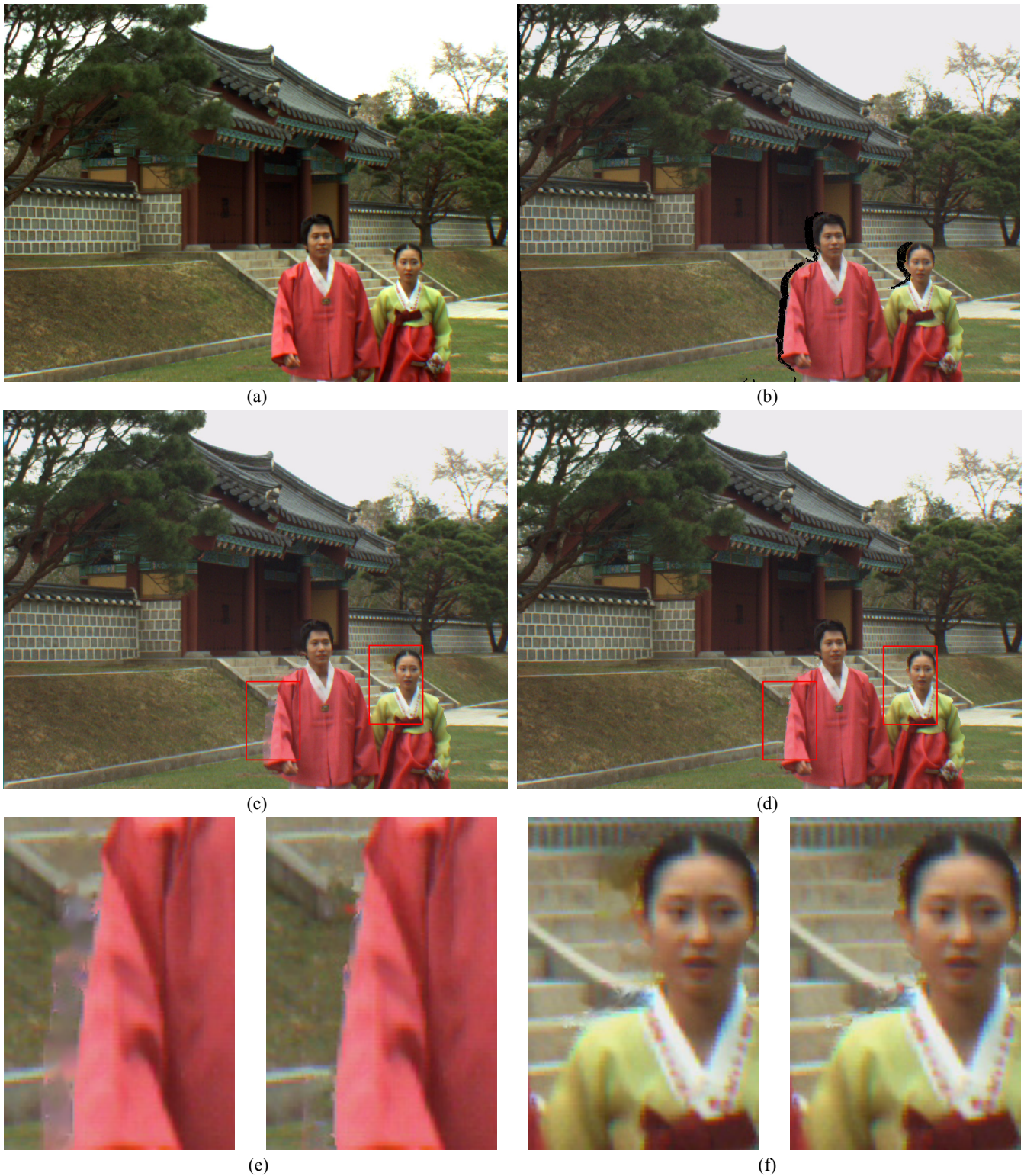
Fig. 5. DIBR results for the sequence "Lovebird1". (a) Original reference image. (b) Warped image with uncovered area marked black. (c) Result of picture 116 by MPEG VSRS. (d) Result of the proposed approach for the same picture. (e) and (f) Magnified results. Left, MPEG VSRS. Right, the proposed approach.
