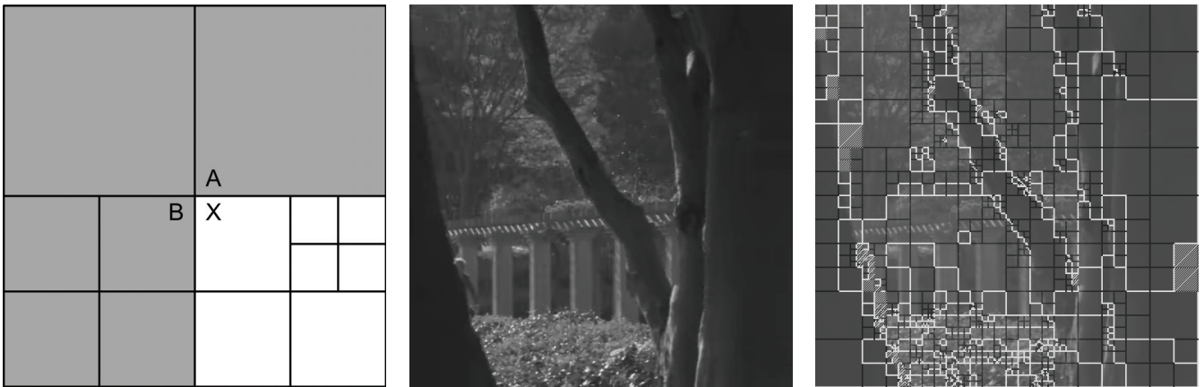
Fig. 2. Left: Schematic representation of a current block X , its set of merging candidates \{A, B\} , and its causal neighborhood (gray shaded). Middle: Cropped part ( 512 \times 512 ) of a frame of the 1080p test sequence “Park Scene”. Right: Illustration of MCP blocks (black lines), merged regions of MCP blocks (white lines), and intra-coded blocks (striped pattern) for the same cropped “Park Scene” content. With a chosen CTB size of 64 \times 64 , an area covering 64 CTBs is shown. Note that “Park Scene” contains a scene captured using a laterally from left to right moving camera and thus, the trees in the foreground, as shown in the middle image, appear to be moving to the left while the background park scene between the trees appears to be (slightly) moving to the right.
